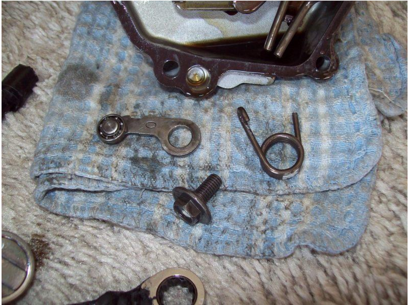
Figure 3 - Detent Lever, Spring, and Retaining Screw
