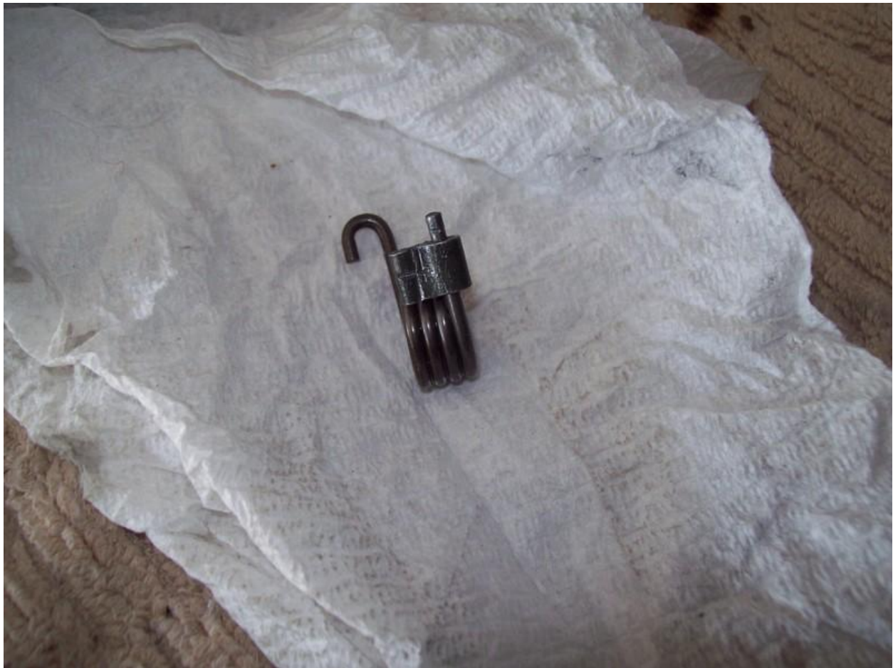
Figure 4 - OEM Spring with Spacer attached
